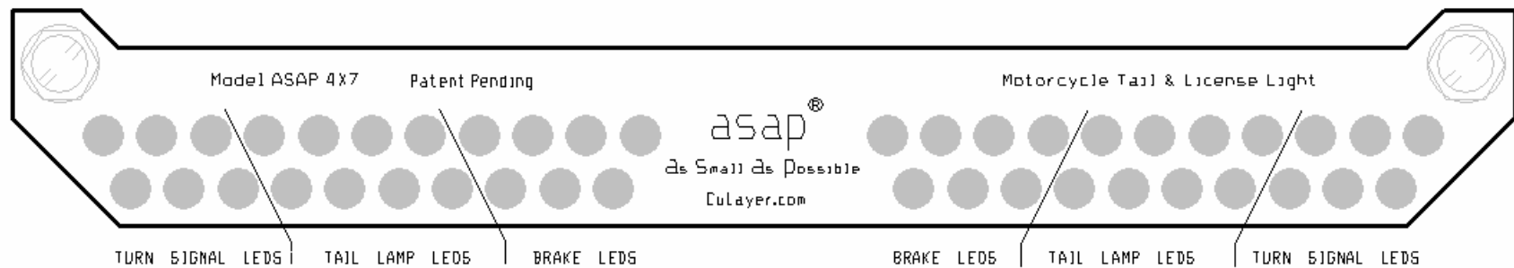
Figure 1: Standard Cover Plate and LED Positions
