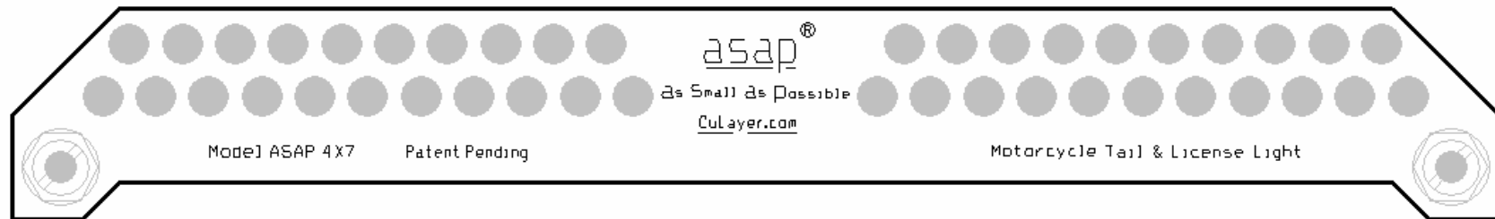
Figure 2: Alternative Cover Plate for Over-the-Top Mounting
